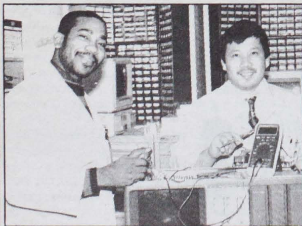
Marvin Campbell (left), biomedical training coordinator and Florante Alfaro (right), biomedical technician check the function of an ECG machine at Children's Memorial Medical Center.
